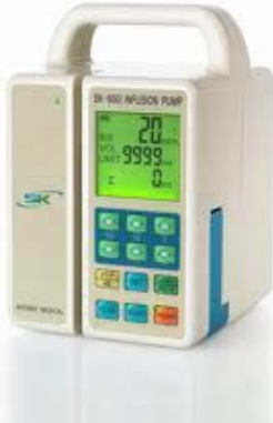
An infusion pump meters out a specified amount of drug therapy over a specified time. Infusion pump recalls are among the highest of all software-based medical devices.
